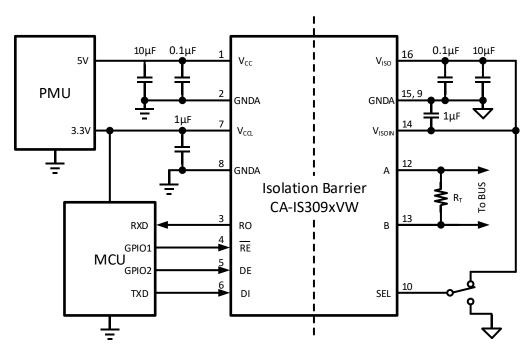
Figure 10-1. Typical application circuit
