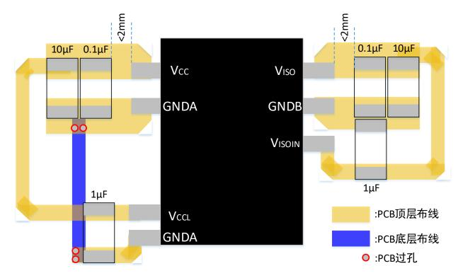
Figure 10-3. Recommended PCB Layout
