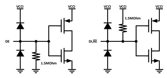
Figure 9-1. Input equivalent circuit
