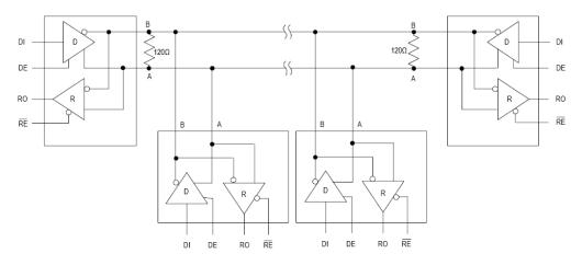
Figure 10-2. Typical isolated half-duple RS-485 application circuit
