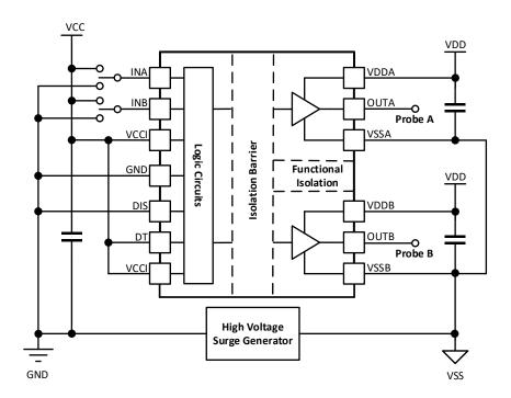
Figure 8-6. Common-mode transient immunity test circuit
