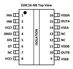
Figure 6-1. The CA-IS3221-Q1 Pin Configuration (SOIC16 Narrow Package)
