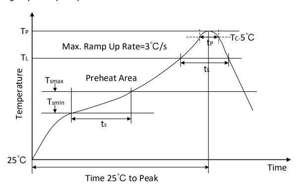
Figure 12-1. Soldering Temperature (reflow) Profile
