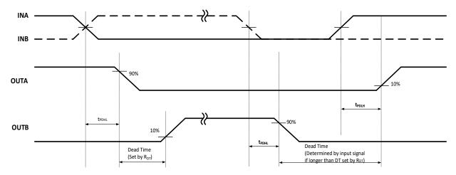
Figure 8-4. Dead-time switching parameters
