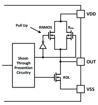
Figure 9-2. Driver output stage
