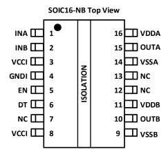
Figure 6-2. The CA-IS3222-Q1 Pin Configuration (SOIC16 Narrow Package)
