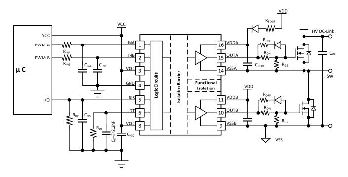
Figure 10-1. Typical application circuit for CA-IS3221-Q1
