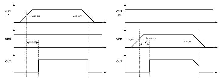
Figure 8-5. VCCI/VDD\_ UVLO power-up delay
