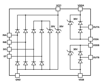
Figure 9-4. ESD protection circuit
