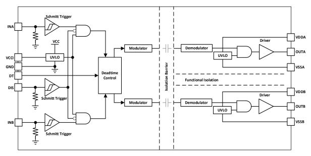
Figure 9-1. Functional block diagram
