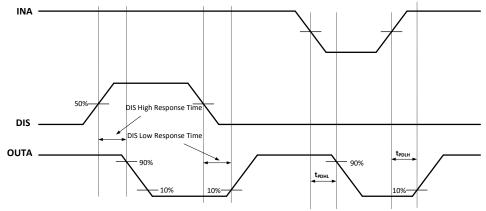
Figure 8-3. Disable timing diagram
