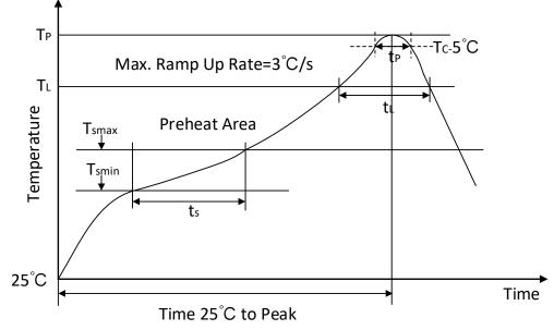
Figure 12-1 Soldering Temperature (reflow) Profile
