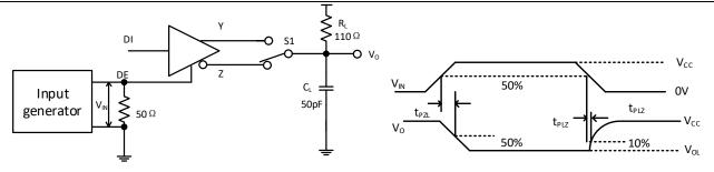
Figure 8-5. Driver Enable and Disable Times With Active Low Output and Pull-up Load
