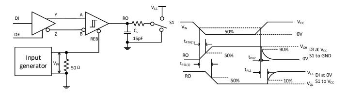
Figure 8-7. Receiver Enable/Disable Times With Driver Enabled
