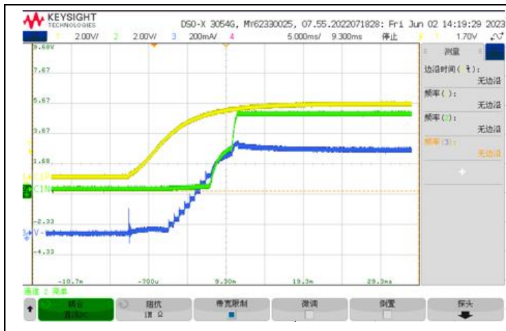
Soft-start waveform: V_{INP}=5V (yellow), V_{ISO}=5V (green), I_{ISO}=300mA (blue)
