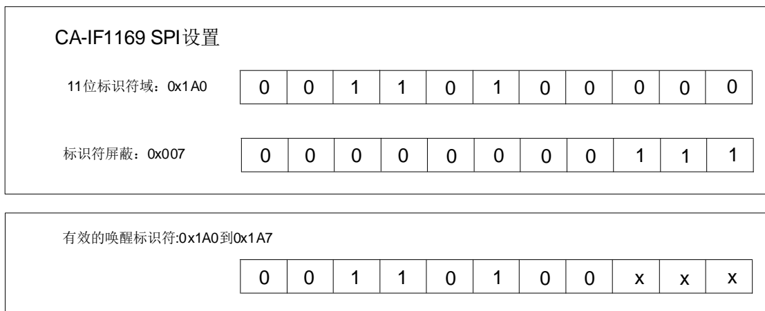
Figure 10-10. Identifier field detection in a selective WUF
