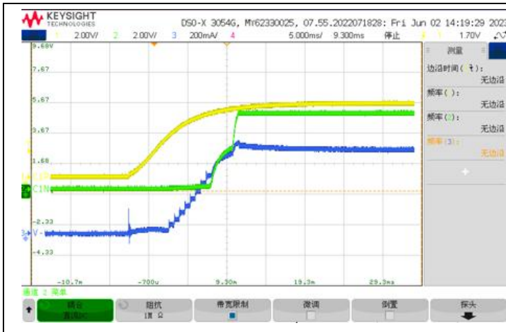
Soft-start waveform: V_{INP}=5V (yellow), V_{ISO}=5V (green), I_{ISO}=300mA (blue)
